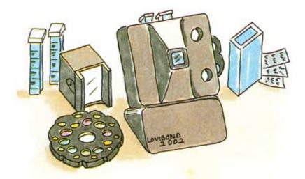
An important point worth mentioning and often overlooked by operators is that for accurate results to be obtained when using this type of equipment, the correct lighting conditions should be used.
