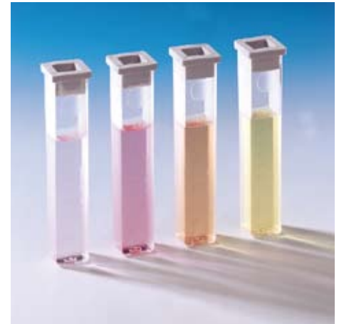
Plastic cells, frosted on two sides, volume 10 ml, path length 13.5 mm, with lids
