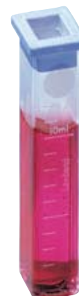
Glass cell with lid, volume 10 ml, calibrated 2 - 12 ml, path length 13,5 mm, Pack of 5, code: 35 42 43
