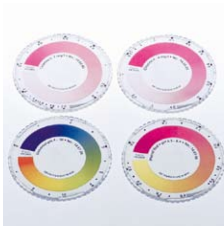
CHECKIT® Discs with continuous and stable scales
