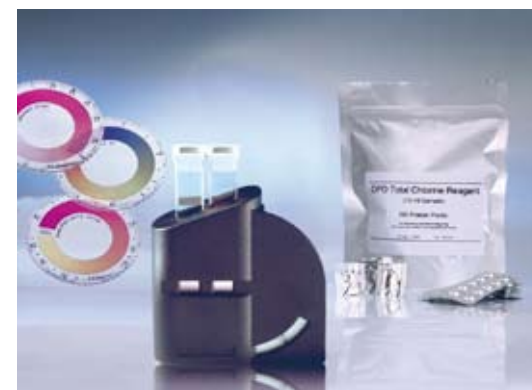
CHECKIT®Comparator with Powder Reagent
