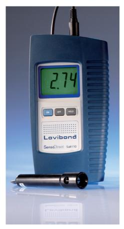
Following many enquiries from customers we introduced the new SensoDirect Salt110 salt tester. Salt content is of great importance in so many applications: pools, thermal baths, brine and mineral baths and in any pools where seawater is used. We recommend regular checks to ensure that salt concentrations do not fluctuate excessively.
