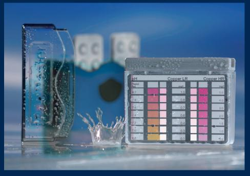
The new, hand-held visual comparator from Lovibond® introduces a new method based on the formation of copper ions.
